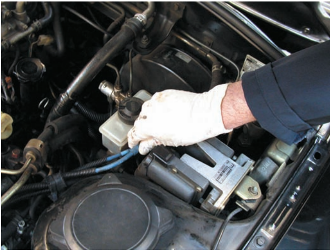
FIGURE 1-3 Protective gloves such as these vinyl gloves are available in several sizes. Select the size that allows the gloves to fit snugly. Vinyl gloves last a long time and often can be worn all day to help protect your hands from dirt and possible hazardous materials.
