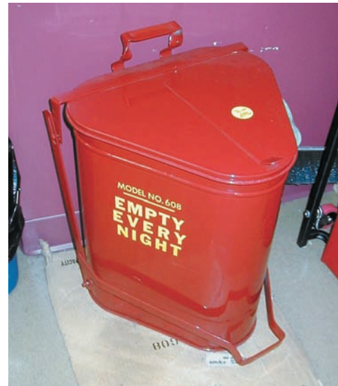
FIGURE 1-9 All oily shop cloths should be stored in a metal container equipped with a lid to help prevent spontaneous combustion.
