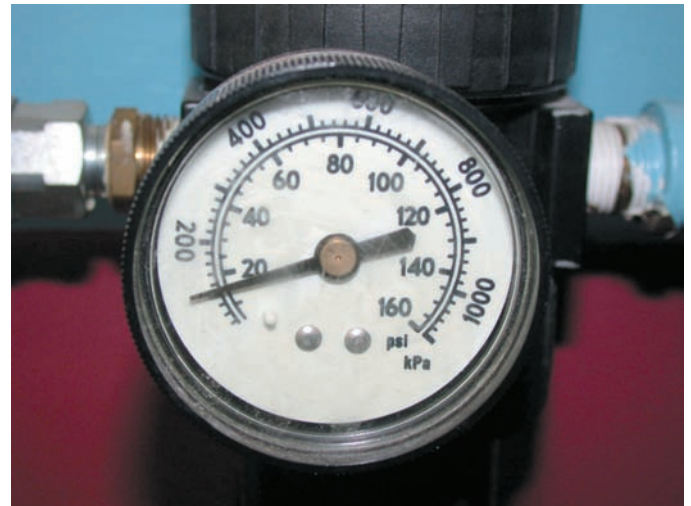
FIGURE 1-11 The air pressure going to the nozzle should be reduced to 30 PSI or less.
