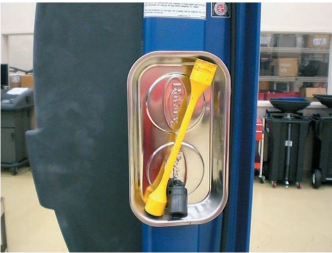
FIGURE 1-7 A magnetic tray is a helpful item to keep tools needed up where they can be easily reached without having to bend over saving time and energy over the course of a long day in the shop.
