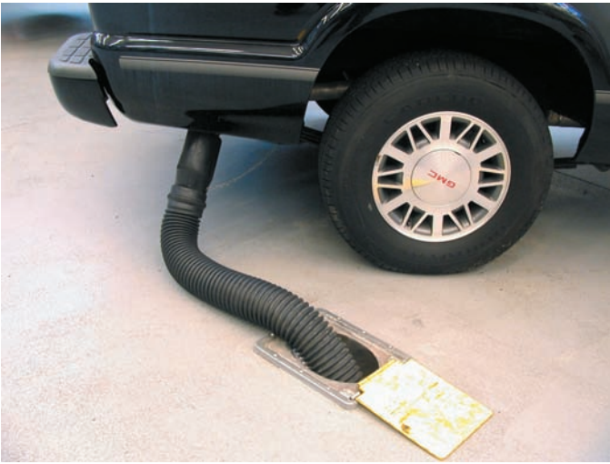
FIGURE 1-6 Always connect an exhaust hose to the tailpipe of the engine of a vehicle to be run inside a building.
