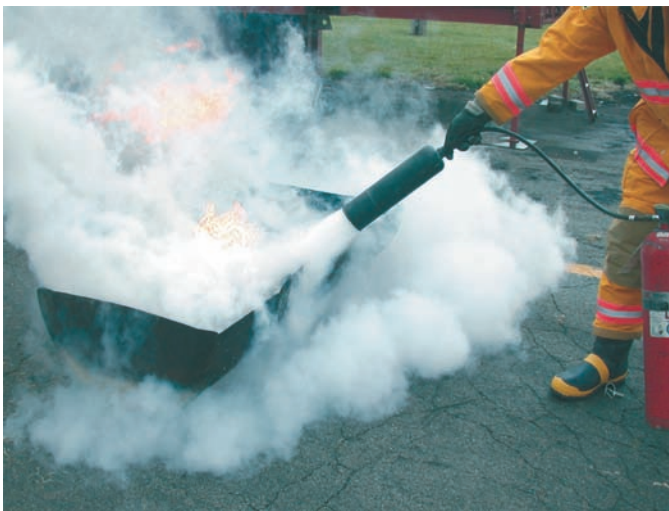
FIGURE 1-13 A CO 2 fire extinguisher being used on a fire set in an open steel drum during a demonstration at a fire department training center.
